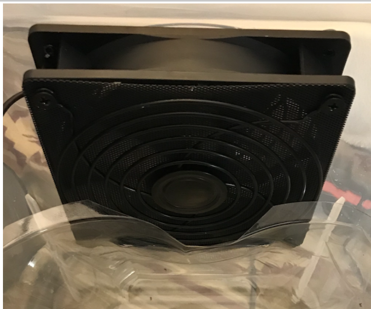
View of the mounted fan from the inside, looking outward. Plastic at bottom is part of the front panel liner that will hold the aquarium pump.
